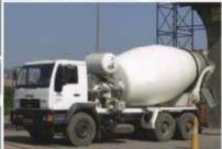
Advantage Schwing Stetter Mixers available with slave engine or PTO drive
