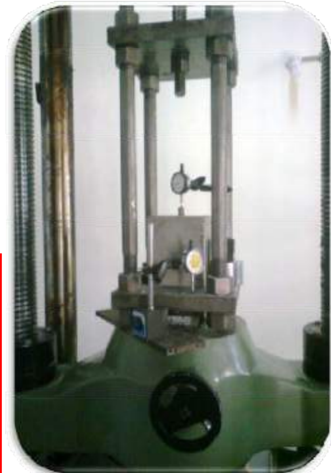
Bond Strength Test
