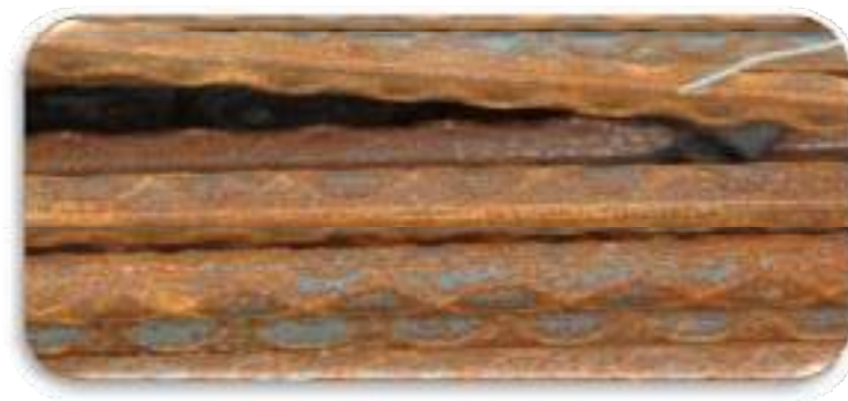
Corrosion of Steel in Water with Oxygen
