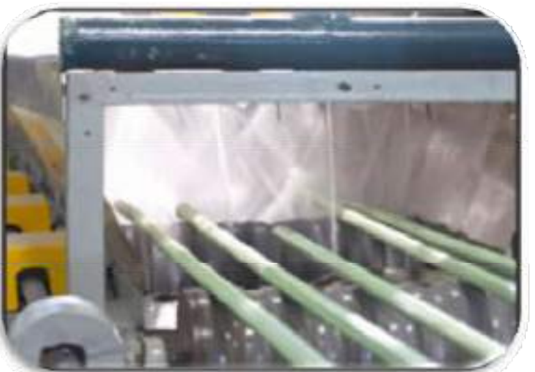
Epoxy Coating – Electrostatic Spray Technique
